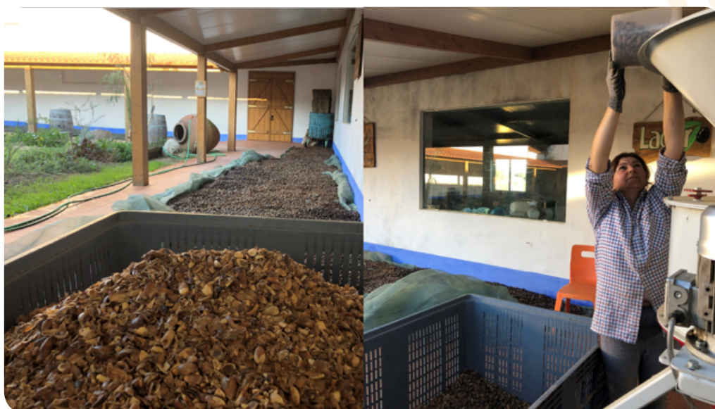
Figure 2. Acorn peel. Acorns are dumped continuously through a funnel and goes by a paddle mill that rotates high speed, breaking it and detaching it from shells. Credits: Cooperativa de Usuários do Freixo do Meio.
